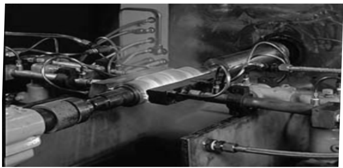
Fig.3. Spin Hardening Of Gear Teeth On Worm Shaft
