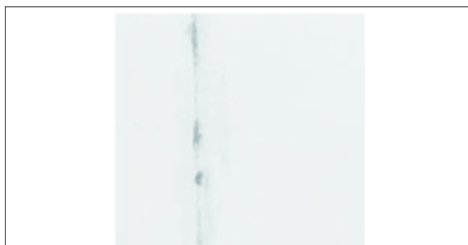
Fig 9: Bending adhesion test fail at low PMT in primer oven. (before optimized temperature.)
