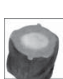
Fig 9: This photograph provided by Dr. C. S. Vishwanath, Bangalore illustrates a highly over-quenched rebar. The hardened periphery is about 60% of the total cross-sectional area. Produced by mill personnel who are not fully trained in quenching & tempering technology. Such bars will have high Yield Strength and very poor ductility and should never be used in civil construction.
