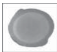
Fig 6: This photograph provided by HSE Germany, illustrates a good Q & T Thermex rebar. Note the uniform and concentric hardened periphery and the softer core. Such bars will have desired tensile strengths coupled with high elongation as required in seismic zones.
