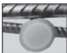
Fig 7: Photo of Thermex rebar provided by HSE Germany. The uniform tempered martensite periphery is clearly visible. Depending on the size and grade, the hardened periphery will be about 20 to 30 % of the bar cross
