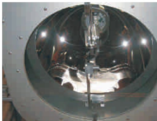
Illumination head of ABB SpectraFlow BM100 online analyzer
