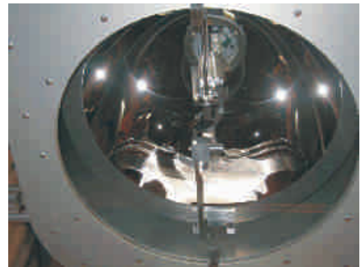
Illumination head of ABB SpectraFlow BM100 online analyzer
