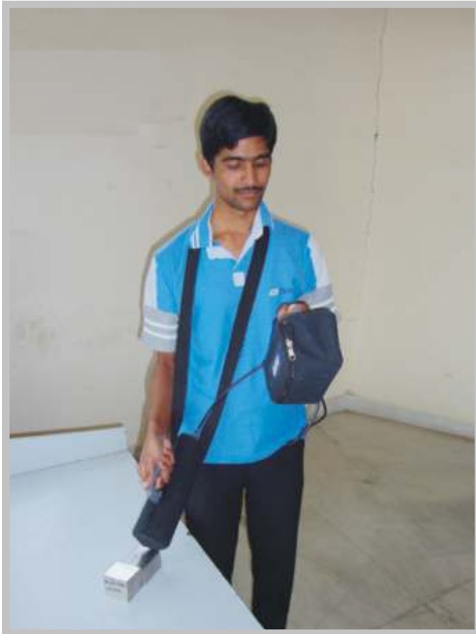
Person checking for radioactive contamination using Rad check meter with external probe
