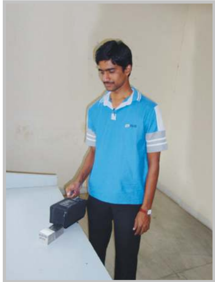
Person checking for radioactive contamination using Rad check meter with internal Detector
