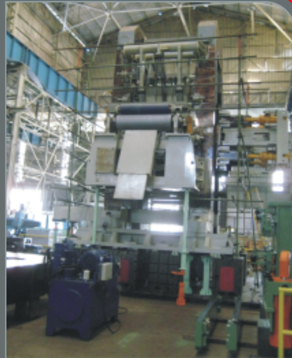
Cold rolling mill under manufacture at CMI FPE Plant at Taloja
